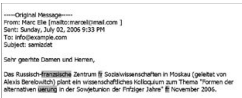
Figure 1b. Diacritical characters distorted or lost due non-matching encoding used by recipient's MUA 5 or operating system.
